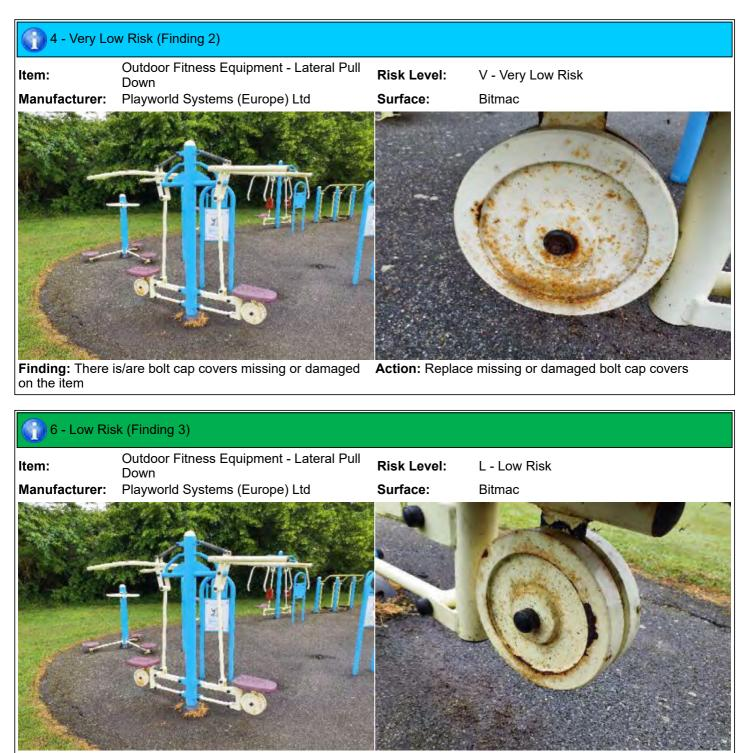
Finding: The paintwork on this item has been damaged or Action: Treat any rusting components and repaint worn exposing the metal underneath which is rusting
