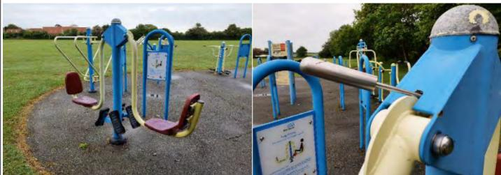
Finding: There are gaps between 8 and 60mm creating a potential crush/shear point in contravention of the requirements of BS EN 16630
