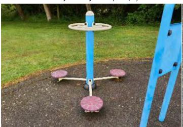
**Finding:** The rotating user station is not appropriately marked with a guideline of user direction and/or the original position as required by BS EN 16630
