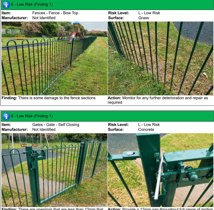
**Finding:** There are openings that are less than 12mm that could trap or crush fingers
