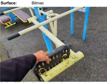
Finding: The swinging movement of the item exceeds the maximum 55 degrees from the vertical required by BS EN 16630
