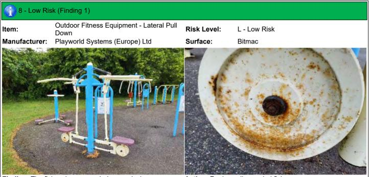
Finding: The fixings have corroded excessively
